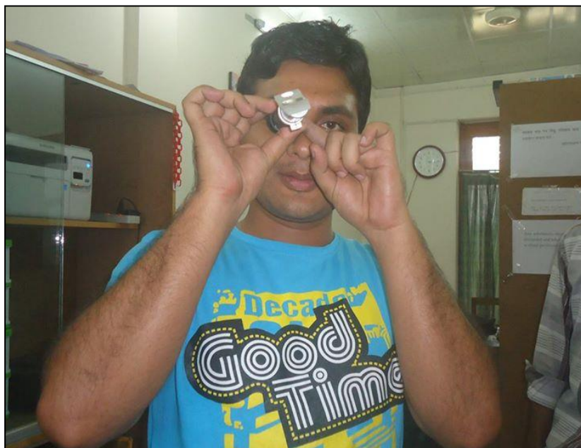
Plate 6 : Photograph showing determination of TSS with Hand Sugar Refractometer
