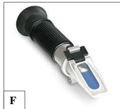
Plate 3. Nutritional analysis in lab A. Determination of pH B .Ethylene determination in hot water bath. C. Titration of tomato juice with dye for vitamin C determination D. development of proline layer. E. Vitamin C determination final point, F. Brix detetrming Refractometer
