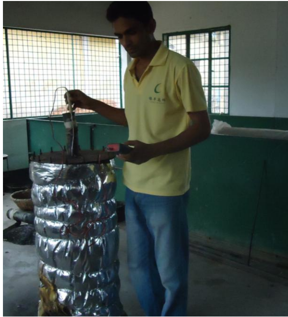
Fig.4.1.6: Measurement of temperature profile of different zone inside the reactor
