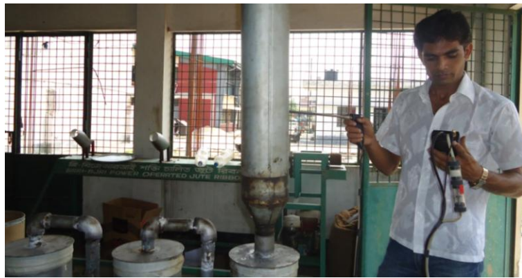
Fig.4.1.4: Measurement of CO and O 2 in the producer gas
