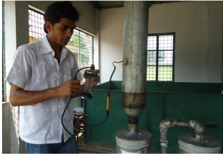
Fig.4.1.3: Measurement of CO 2 in the producer gas
